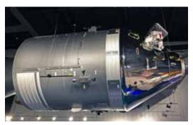
that supplies oxygen, water, electrical power, communication, and propulsion for the spacecraft, and is jettisoned just before reentry.
